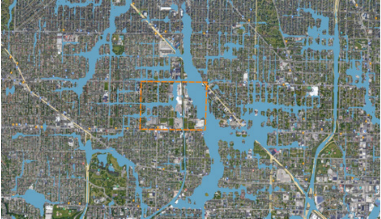
FIGURE 21: Pluvial flooding in Metcalfe Park under an extreme precipitation scenario (a 100-year, 1-hr storm). Flooding is considered when the maximum flood depth obtained during the simulation exceeds 4 inches.
